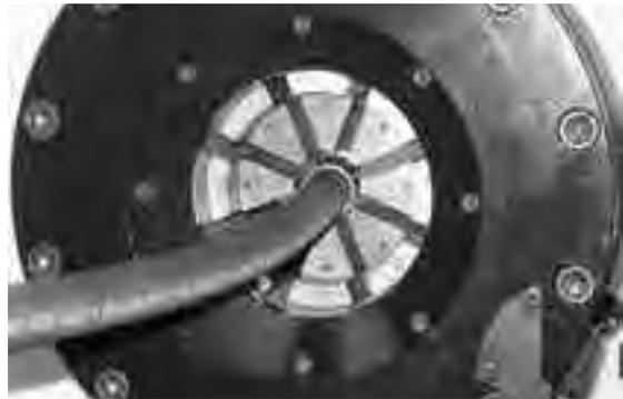
Insert hose assembly into crimper die set.
