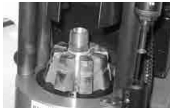
Insert hose assembly into crimper die set.
