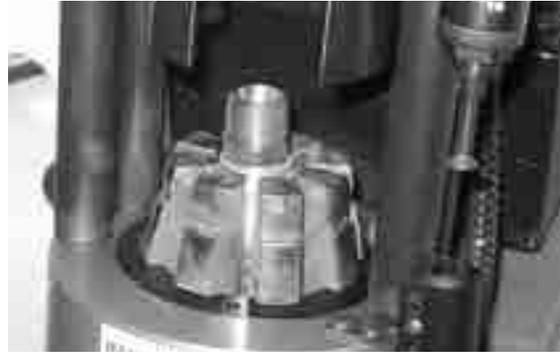
Insert hose assembly into crimper die set.
