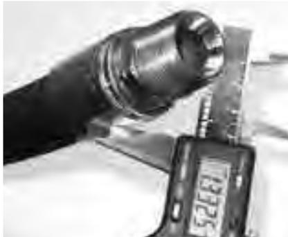
Verify crimp diameter with calipers.
