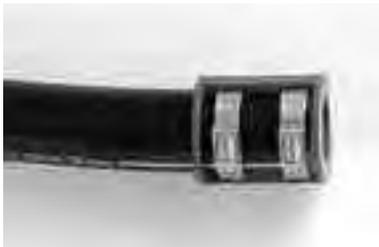
5. Insert the fitting into the hose. Ensure that the fitting is fully inserted so that there is no gap between the end of the hose, the clip retainer and the shoulder of the fitting.
