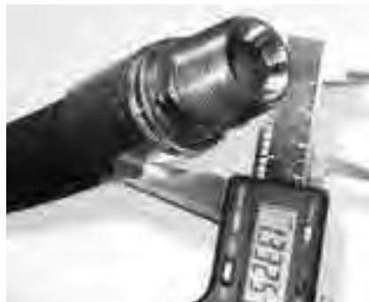
Verify crimp diameter with calipers.
